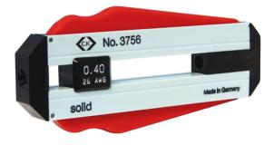
Features & Benefits  $\sim$  Compact precision wire strippers for repeatable, damage free stripping of PVC, Teflon & similar coated wire  $\sim$  Graduated depth stop for stripping to precise lengths  $\sim$  Specially hardened blades for outstanding long term performance  $\sim$  50 mm scale with 1 mm graduations and length stop  $\sim$  For diameter: 1,00 mm (18 AWG)
